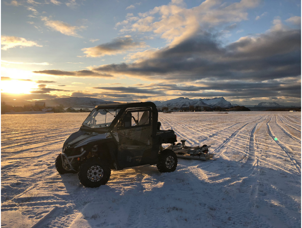
Fig. 1. Performing a ground-penetrating radar survey in Northern Norway. Photo: Arne Anderson Stamnes.
